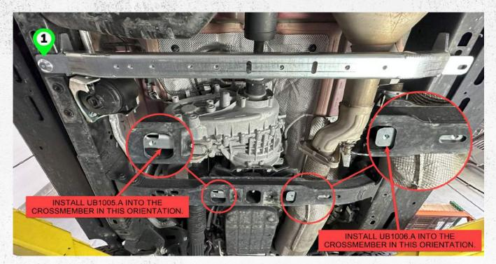
Step 10. <u>Loosely</u> install the provided crossmember using 1- M12 x 40 flathead bolt with the tapered washer **①** as shown above. Insert the 2 nut plates as shown above.
