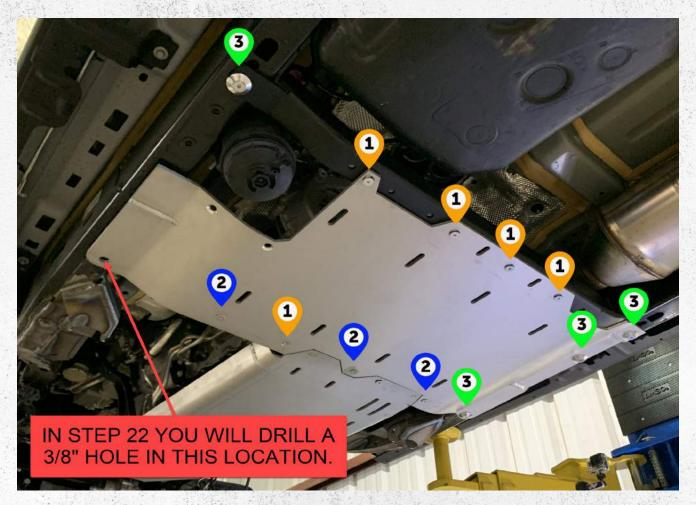
Step 12. Continue by <u>loosely</u> securing T-case skid onto support crossmember using  $5 - 3/8 \times 1^n$  counter sink bolts 0, and  $6 - M12 \times 40$ mm bolts 0/0 using the 0/0 allen wrench. Octains also use a tapered washer.
