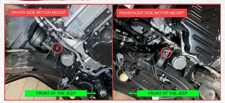
Step 8. To install the motor mount skid brackets, first remove the factory 10mm bolts from these two locations (RED) circled
