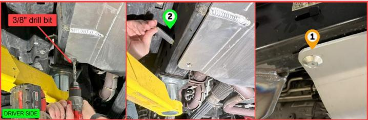
Step 21. Once the skid plates are tightened, drill a 3/8" hole in the necessary location(s)
