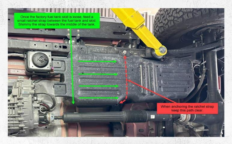
Step 6. Using a small ratchet strap you will suspend the tank so that you can remove the factory fuel tank skid. Make sure to anchor the ratchet strap to something substantial. After suspending the tank you can remove the fuel tank skid. This can take some time, and can be frustrating but it is necessary. For easiest removal, it helps to have less than 1/4 tank of fuel, as noted in the SPECIAL NOTES on page 2.
