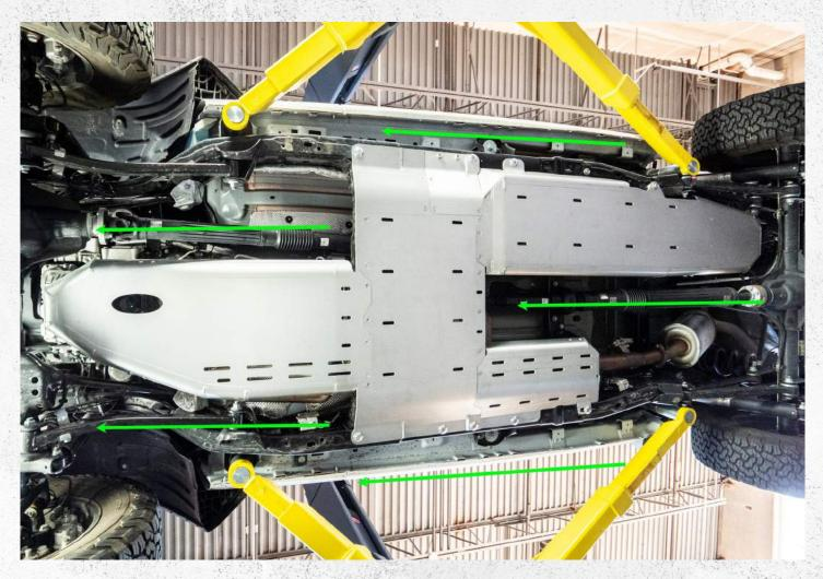
Step 20. Starting from the rear of the vehicle while working your way forward to the front end, tighten/torque all skid and bracket hardware that was previously loosely installed on fuel tank skid, T-case skid, and engine oil skid.
