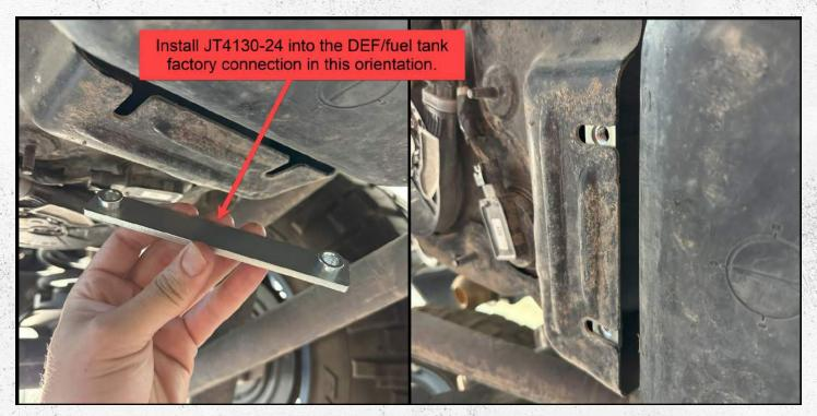
Step 15: Install JT4130-24 as seen above. Make sure the surface is clean before installing.
