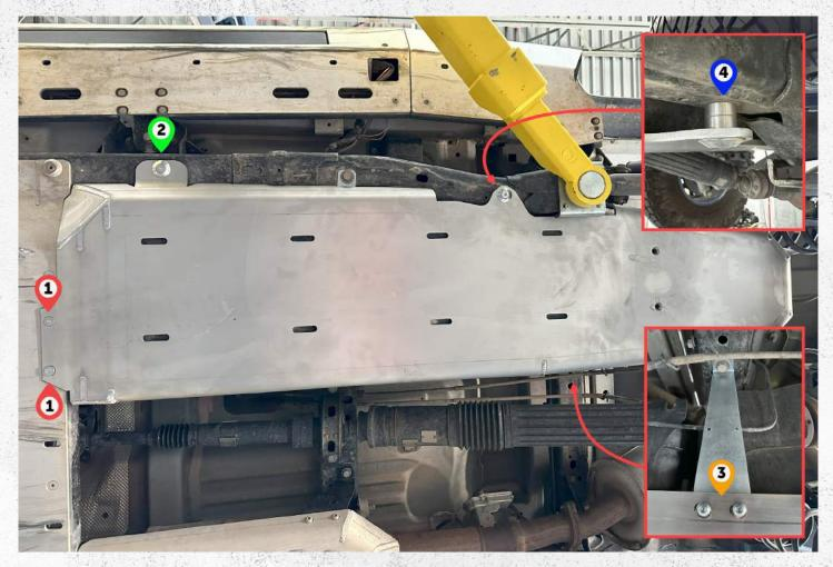
Step 16. Using the 7/32 Allen wrench <u>loosely</u> assemble the gas tank skid with 2 – 3/8 x 1" flathead bolt 1, 1 – M12 x 40mm flathead bolt with tapered washer 2 AND 2 – 3/8 x 1" buttonhead bolts with 3/8 flat washers 3. At location 3 assemble using 1 – M12 x 40mm flathead bolt with tapered washer AND 2 of the 10mm machined aluminum spacers as seen above. You will need to use a jack/lift to press the skid close enough to the frame to install the hardware and spacers.
