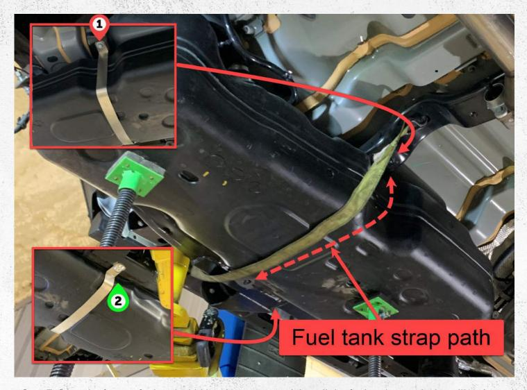
Step 7: Once the factory fuel tank skid has been removed, install the fuel tank strap by installing 1 - OEM 12mm bolt 1 with a 18mm socket AND 1 - 12mm x 40mm counter sink bolt & counter sink washer 2 using the 7/32 allen wrench. The fuel tank strap hardware can be tightened at this stage. Once the fuel tank strap is mounted you can remove the ratchet strap.
