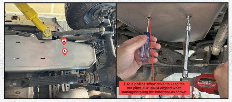
Step 17. Using the 7/32 Allen wrench <u>loosely</u> install 2 − 3/8 x 1.5" flathead bolt **1** into the previously installed nut plate JT4130-24.
