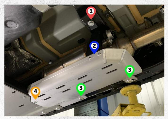
Step 14. <u>Loosely</u> install the exhaust skid with  $1 - 3/8 \times 1$ " flathead bolt 0,  $3 - M12 \times 40$ mm flathead bolts with tapered washers 0 and  $2 - 3/8 \times 3/4$ " buttonhead bolts with flat washers 0 using the 7/32 Allen wrench. Use the OEM M12 bolt 0 in this location.
