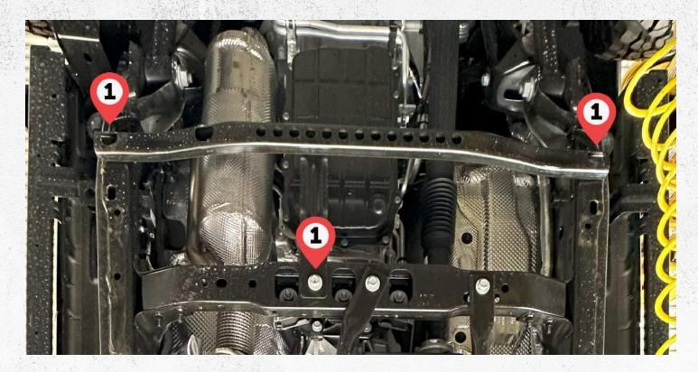
Step 3: Remove the transmission skid by removing 3 − 12mm bolts 0 using a 18mm socket.
