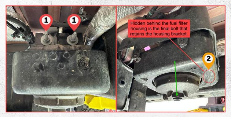
Step 2: Remove the fuel filter housing bracket by first taking the 2 – 8mm nuts **0** off using a **1**3mm deep well socket. Once the fuel filter housing is free, push it upward far enough to allow access to the **1** – 8mm bolt **2**, using a **1**3mm socket. NOTE: having a swivel here makes removing that bolt easy.
