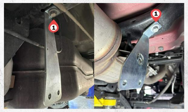
Step 13: <u>Loosely</u> install both the fuel skid and exhaust skid inner brackets as shown above using 2 - 12mm OEM bolts 1 with a 18mm socket.
