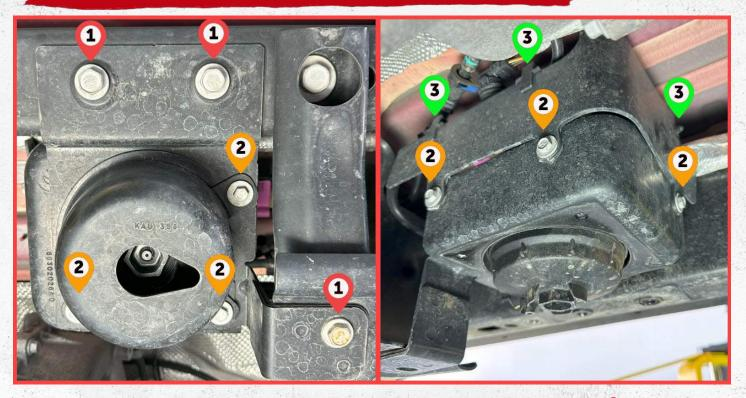
Step 1: From left to right: Disassemble the fuel filter skid by removing 3 – 8mm bolts ① using a 13mm socket AND 3 – 5mm bolts ② with a 10mm socket. Once the fuel filter skid is out of the way, remove the plastic shield by first disconnecting the plastic Christmas tree tabs ③ from the plastic shield. Then remove 3 – 5mm screws ② using a 10mm socket. Keep 2x ① OEM hardware.
