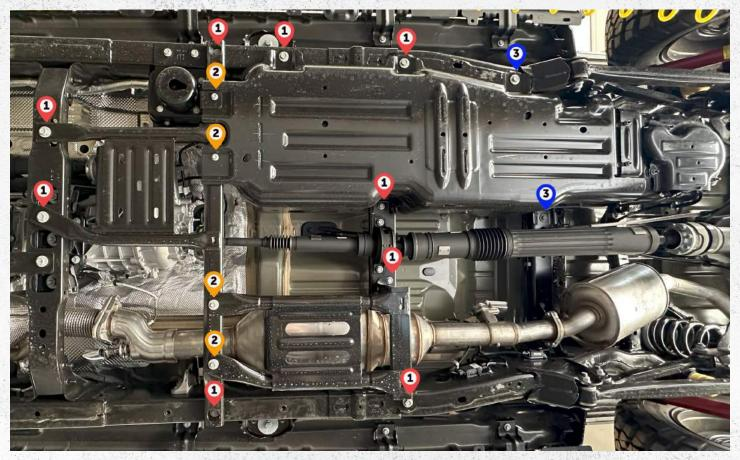
Step 5: Remove the transfer case & exhaust skid by removing 4 - 8mm bolts ② using 13mm socket AND 8 - 12mm bolts ① using a 18mm socket. Loosen but do not remove 2 - 12mm bolts ③ using a 18mm socket.
