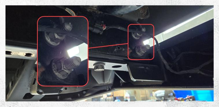
Step 2: Use a 21mm socket and wrench to remove the two factory bolts on both sides of the vehicle.
