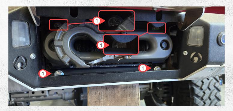
Step 2: Install the grade 8 hardware RED 1 through the bracket using the winch nuts to secure it to the high clearance bumper.
