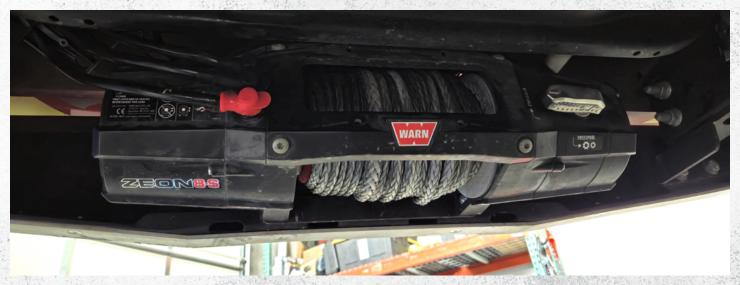
Verify ALL previously installed hardware is tight / torqued to specifications.
