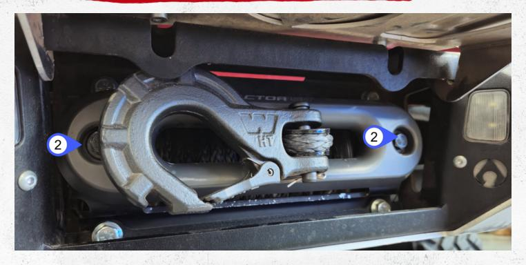
Step 3: Install your fair-lead onto the winch using BLUE 2 and tighten all components.
