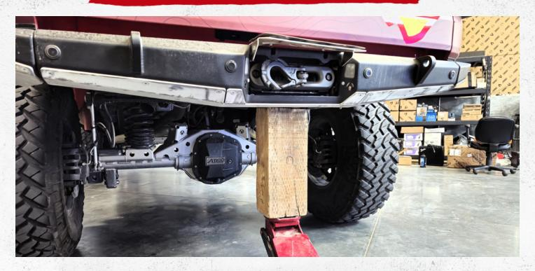
Step 1: Use a jack or other means to align your winch and winchplate to the high clearance bumper.
