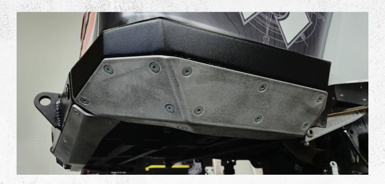
Step 13. With the bumper fully assembled and in the correct position centered in the vehicle, tighten all hardware and re-secure your wiring to the vehicles harness.
