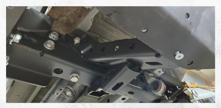
Step 10. Install bracket **JT0120-11 driver side & JT0120-12 passenger side** loosely into position over the corner-pods and aligned with the frame-side brackets **JT0117-20 & JT0117-21**
