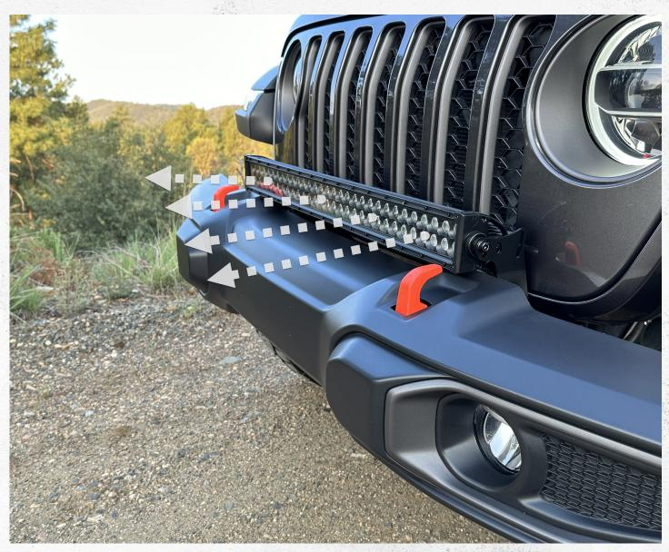
Step 4: With the bracket hardware tightened, adjust your light bar and tighten it per the light manufacturer instructions.
