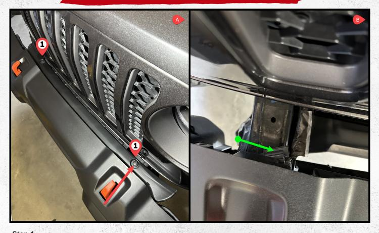
A: Using a screw driver remove the Closeout panel by removing the 2 - plastic push pin rivets
