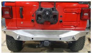
STEP 8. Reuse the four 14mm long frame bolts to fasten the bumper threaded clevis holes to outside of the frame. The top hole can be accessed directly from the side with a normal socket (diagram 4). The bottom hole is accessed using the socket directly on the bolt head and then running an extension through the hole on the side of the bumper and connecting to the socket (diagram 5).
