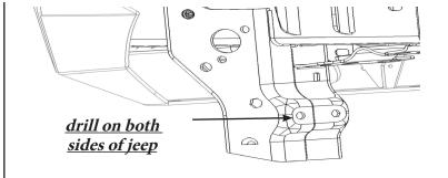
**STEP 3.** Next hold the skid up and loosely install all the hardware. Once all the hardware is installed perform final tightening. If you have not already coated the skid with paint or powder coat we recommend doing this now the fitment is verified.
