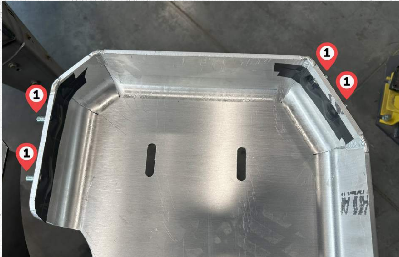
Step 13. Using tape secure 4 - 3/8" x 1" carriage bolts ① to the fuel tank skid prior to installing the fuel tank skid onto frame and support crossmember. Electrical tape works well.
