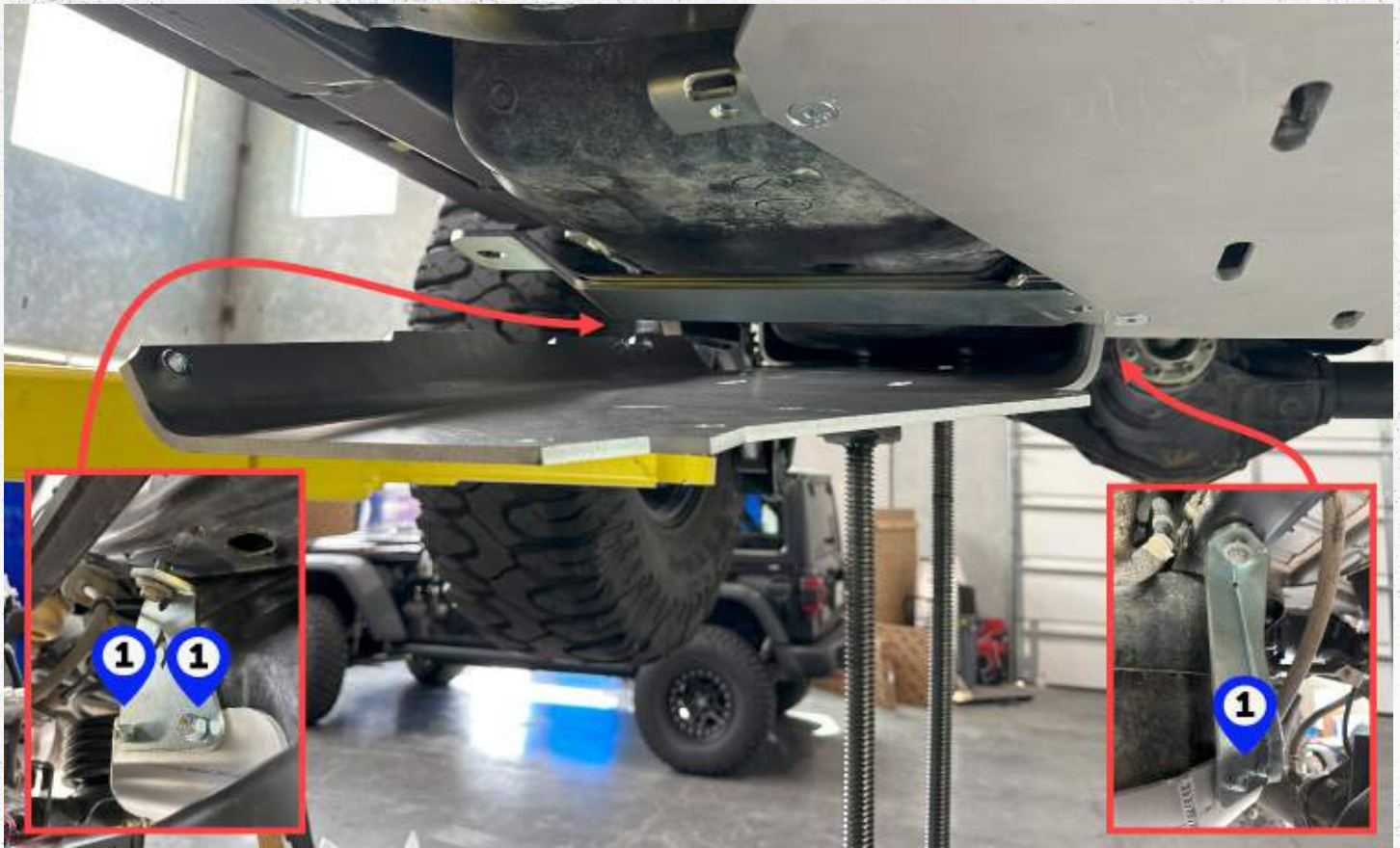
Step 14. Using a 9/16 inch wrench/socket loosely assemble the gas tank skid with 4 - 3/8 x 1" flat-head bolt ①.
