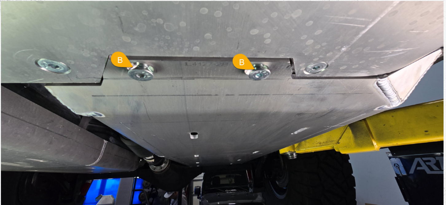
Step 16: Install two 3/8" countersunk bolts.
