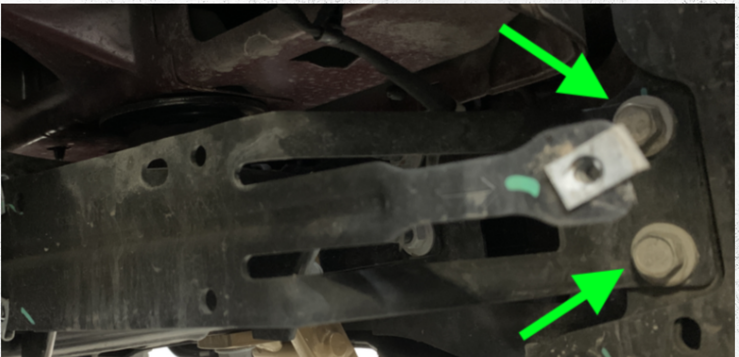
Step 8. Using 16mm socket, install rear bumper side support bracket onto bumper using 2 – OE 8mm bolts from frame side. Repeat to PSG side.
