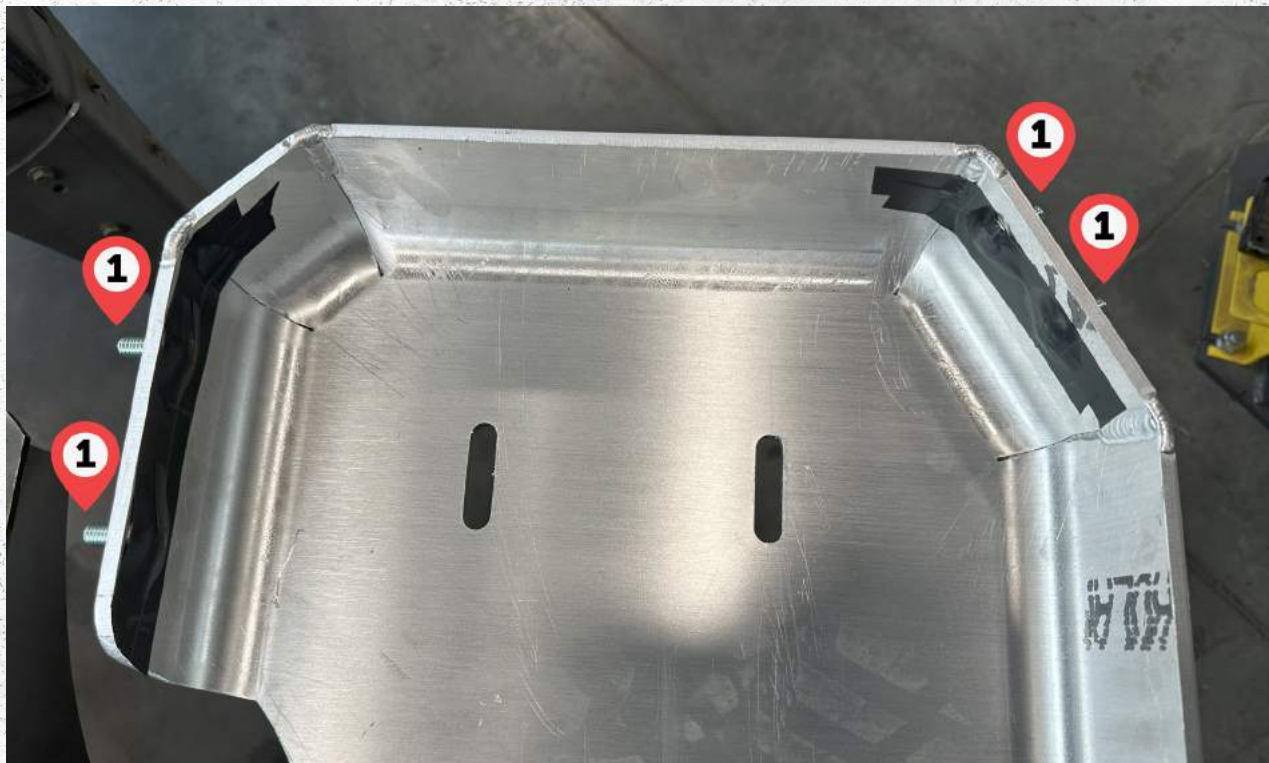
Step 11. Using tape secure 4 - 3/8" x 1" carriage bolts ❶ to the fuel tank skid prior to installing the fuel tank skid onto frame and support cross member. Electrical tape works well.
