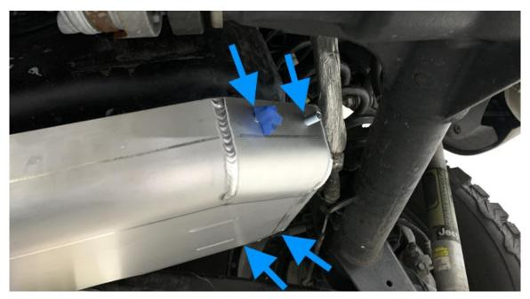
11. **Loosely** installing fuel tank skid onto passenger frame using 3 - 12mm x 40mm countersink bolts and washers. (Green)
