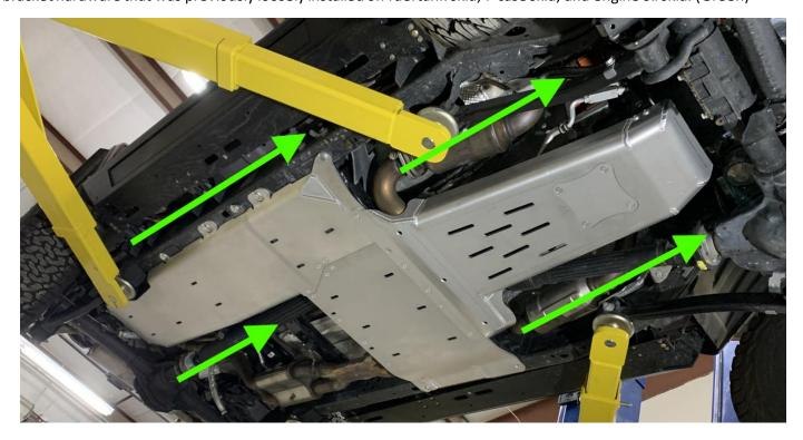
25. Continue by drilling 3/8" hole into driver's side frame rail as shown below. (Green)
