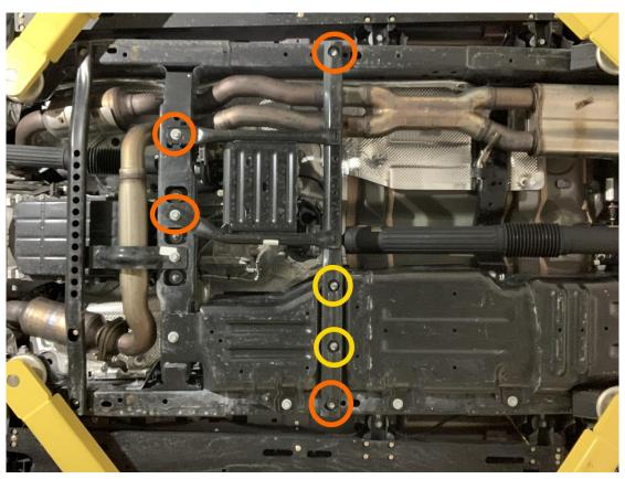
3. Remove fuel tank skid by loosening 5 - 12mm bolts using 18mm socket. (Red) Loosen 2 - 12mm bolts using 18mm socket. (Yellow) Remove fuel tank support strap by loosening 8mm bolt using 13mm wrench. (Orange)
