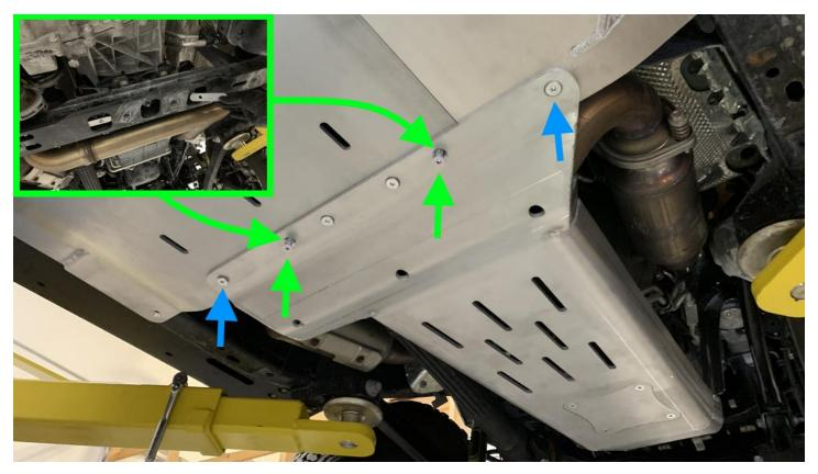
24. Starting from the rear of the vehicle while working your way forward to the front end, tighten/torque all skid and bracket hardware that was previously loosely installed on fuel tank skid, T-case skid, and engine oil skid. (Green)
