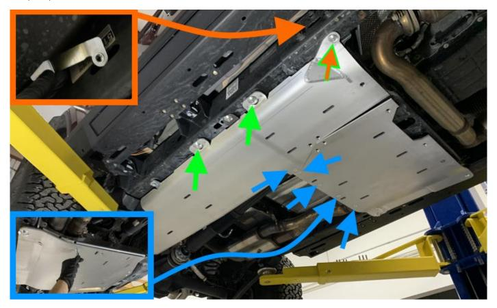
13. Continue by <u>loosely</u> securing T-case skid onto support crossmember using 4 – 3/8 x 1" counter sink bolts. (Green)
