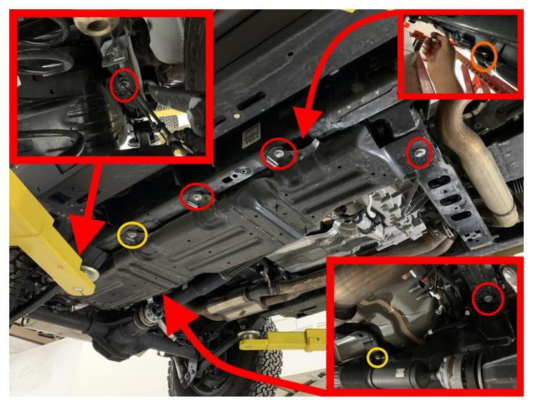
4. With fuel tank skid loosely secured, slip a small ratchet strap between the fuel tank and the fuel tank skid securing the fuel tank to the frame so the OEM fuel tank skid can be fully removed. (Detach clip holding fuel lines to fuel tank skid.)
