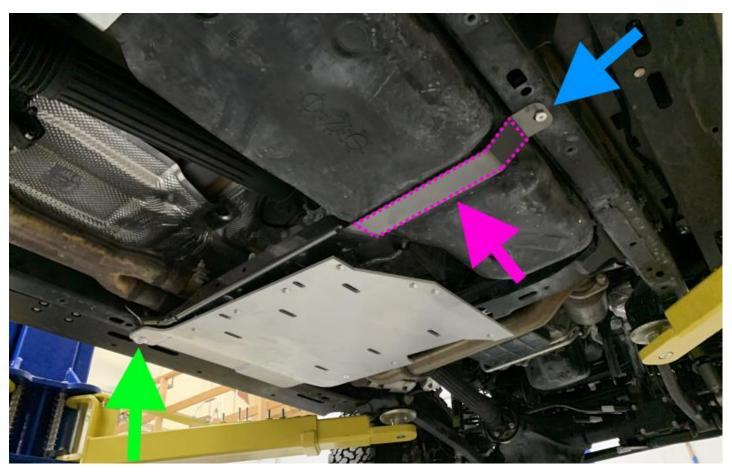
10. <u>Loosely</u> install  $4 - 3/8" \times 1"$  carriage bolt using tape to secure them to the fuel tank skid prior to installing the fuel tank skid onto frame and support crossmember. (Blue)
