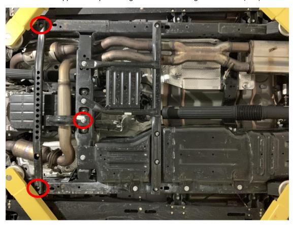
2. Remove transfer case skid by removing 2 - 8mm nuts using 13mm socket (Yellow) and 4 - 12mm bolts using 18mm socket. (Orange)
