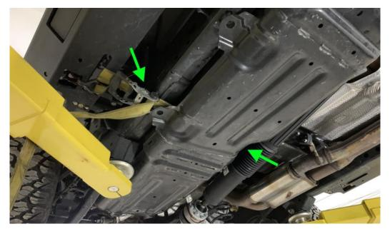
5. With fuel tank secured, install fuel tank strap using OEM 1 - M12 bolts, previously removed, with 18mm socket (Green); 1 - 12mm x 40mm counter sink bolt & counter sink washer through strap and into passenger side frame rail as shown. (Blue)
