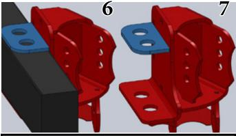
Jeep TJ or YJ - Line up the bolt holes on the bracket with the U-joint of the transfer case yoke, so that the control arms pivot at the same point of the drive shaft.
