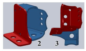
**<u>Step 4</u>**: Install BR1013-16 with a joint between it and BR1013-15. Tack weld in place.
