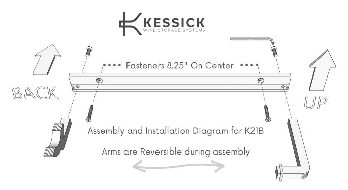
Includes screws and wrench to assemble the arms as well as 1" wood screws to secure the Kessick Wine Hardware a wood surface.
