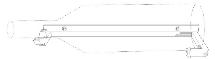
The Kessick Wine Hardware displays wine in a label forward format with the orientation of the wine bottle tilted optimally to maintain constant contact between the wine and the cork. Patent Pending.
