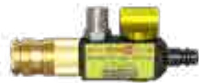
INLINE RELIEF VALVE FOR G2 165 psi / 11.4 bar Designed to relieve over-pressurization and allow a lift bag to remain inflated under a load. This valve will relieve excess pressure from an inflated bag caused by load shifts or temperature changes. Now with safety coupling. Net Weight: 1.0lb 0.4kg Part No. 22-890490-150
