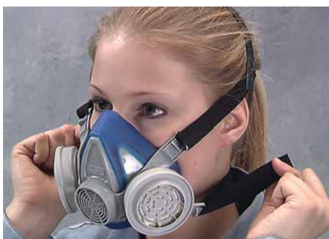
7 - Adjust the cradle headband and neck straps for a comfortable and secure fit.
