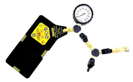
2. Connect the garden hose to the water inlet on the Modular Pressure Director as shown. Open the shutoff valves in front of the hose and gauge then turn on water and fill to house pressure.
