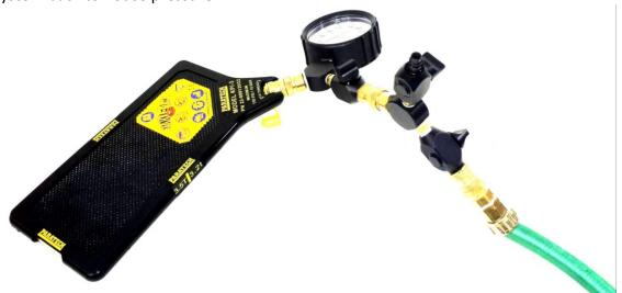
4. Connect the pump assembly to the Modular Pressure Director as shown.
