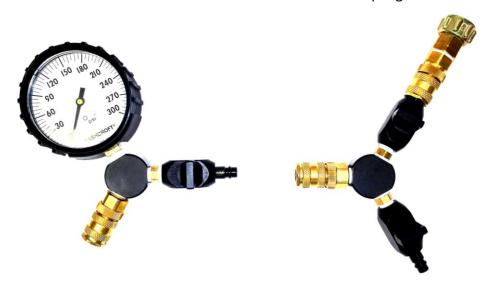
2. Insert the Modular Pressure Director shutoff nipple, gauge side, into the outlet side of the Deadman controller and tighten the coupling lock ring. NOTE: make sure the shut-off valve is in the closed position as shown.
