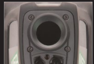
Field-Replaceable Germanium Lens
