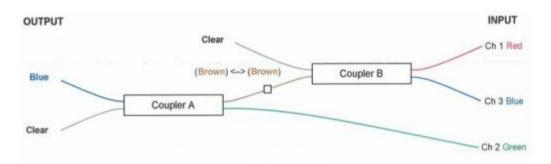
Input 1 1465 nm Red Input 2 1480 nm Green Input 3 1495 nm Blue Output - Blue
