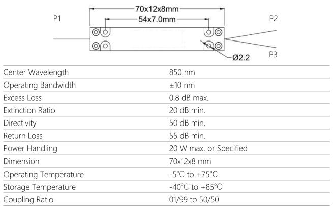
\* With connectors, the handing power is 1 W only, IL is 0.3 dB higher, RL is 5 dB lower, and ER is 2 dB lower.
