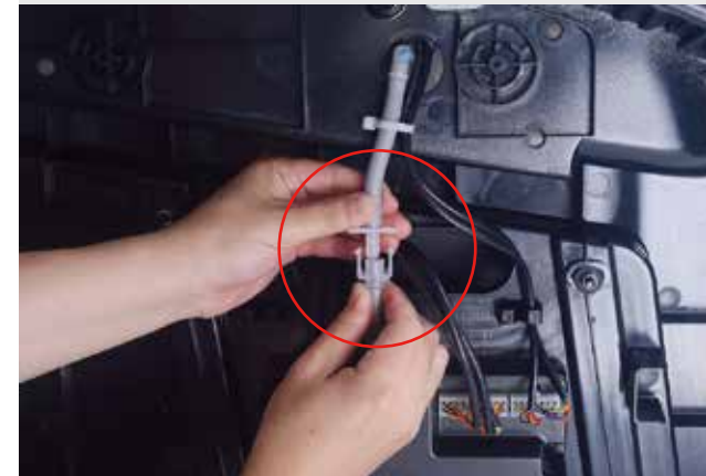
Here is the one way air hose.
