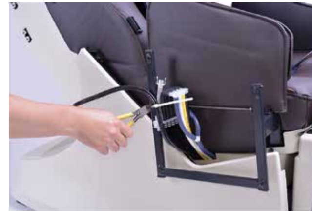
Here is the cable tie you are to cut off.
