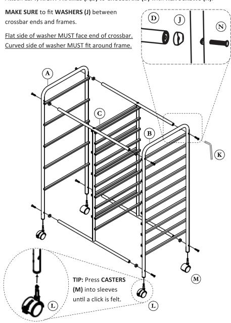
Press LOCKING CASTERS (L) and CASTERS (M) into the sleeves installed in STEP 1.
