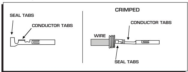
Figure 1 Installing the Terminals.
