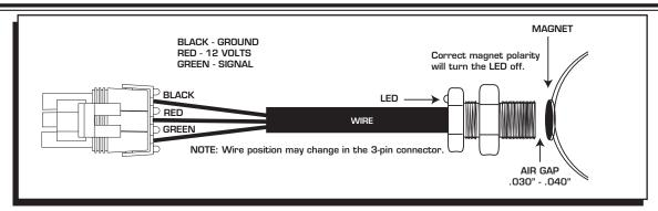
Figure 2 Installing the Hall-Effect Pickup.
