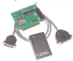
The PIO-12 board requires an available ISA expansion slot in your PC. Before proceeding insure that your PC has an available ISA slot. Some PC's only have PCI expansion slots and cannot be used with the PIO-12 expansion board.
