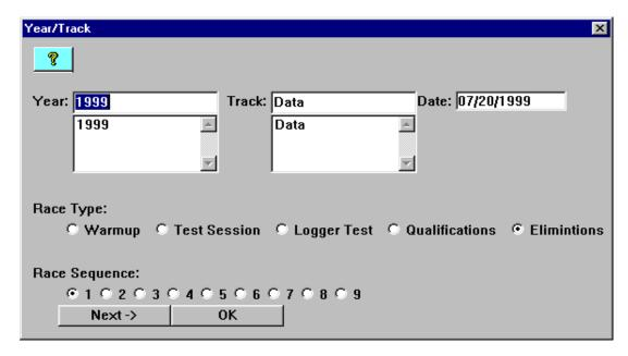
This screen is used to enter the race track and run information used to name and store the run data file. Enter the correct year and track information and select the race type and sequence number with the selection buttons. If the correct year and or track name does not appear in the selection list simply type the correct entry in the selection box. The entry will be added to the selection list and will appear the next time you upload.
