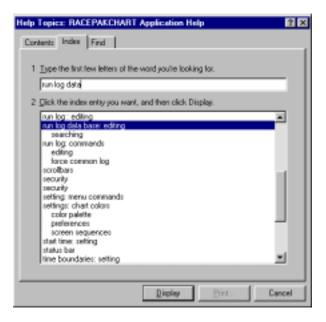
This dialog box allows the user to search the index included with the DataLink help systems for keywords relating to topics that you wish to explore. Type in the word you are looking for in the top line of the dialog box. Entries in the help index beginning with the letters typed in the top line will be displayed as you type.
