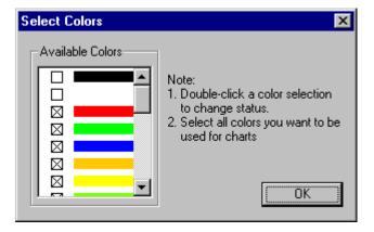
If the box next to the color bar is checked the color is active and will be used in graphing the channels on the display screen. If it is not checked the color is inactive and will be not be used. Using the scroll bar on the available colors box to review the color palette and turn off any colors that do not graph clearly.
