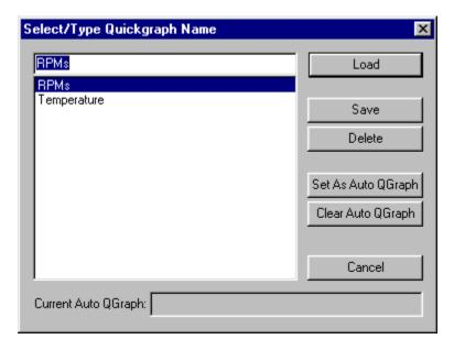
If this is new quick graphs set, enter a name under which to store the graph set in the text entry box on the top and select the **SAVE** button to store the graph set. If you wish to store the graph set under an existing quick graph name, click on the name in the list and then select **SAVE**.
