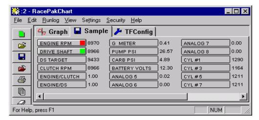
Next find the name of the channel to be edited in the channel buttons located in the channel display pane. Move the mouse cursor over the button and right click on the channel button. The Easy Edit dialog box appropriate for that channel will be displayed. The easy edit dialog box is then used to edit the information on the channel. The different Easy Edit dialog boxes are discussed below.
