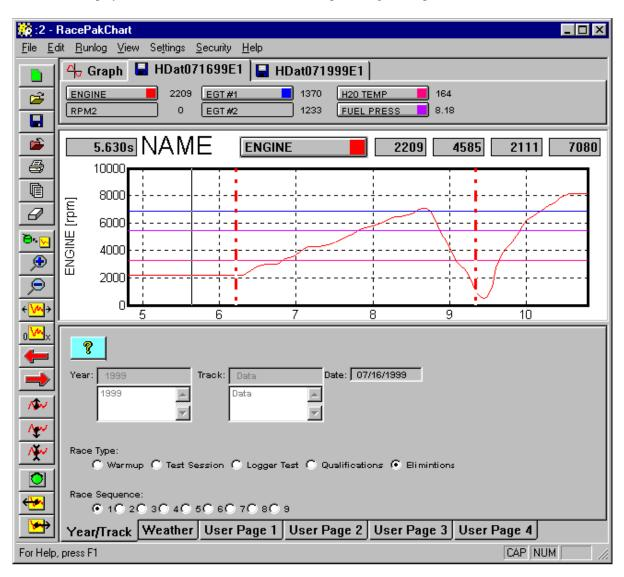
The top region or pane is called the *Channel Display*. This region is used to display the channel control buttons and the numeric data associated with each of the data channels.
