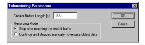
The first parameter **Circular Buffer Length** is used to set the amount of data to record in seconds. The **Recording Mode** is used to determine whether the recording will stop when the maximum record time is
