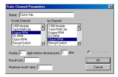
3) Right mouse click on the channel captioned **Spare Ratio3**. Edit the box to match the sample shown below. Select **OK** when finished.
