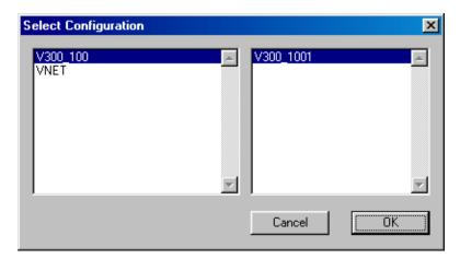
The left-hand column contains a list of the data loggers currently setup in the RacePak DataLink software system. The right hand column displays the list of available configuration files for the highlighted data logger.
