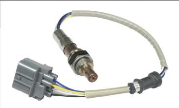
The **NTK UEGO** (Universal Exhaust Gas Oxygen) sensor is a 5 wire wideband Lambda sensor. It is used to control fuel and ignition systems to optimize a car's performance in the areas of emissions and fuel economy.
