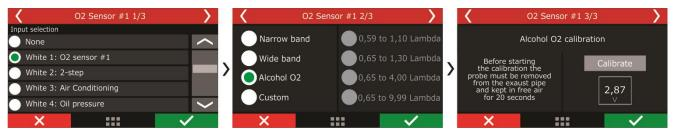
The free-air calibration also can be performed through FTManager Software. To reach the calibration screen, with an open map, go to **Sensors and Calibration** in the left menu, then enter **Inputs** and select the channels where the Alcohol O2 analog outputs are connected.
