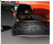
**Double ball bearing wheels** Ensures the mower rolls easily, even after many years of use.
