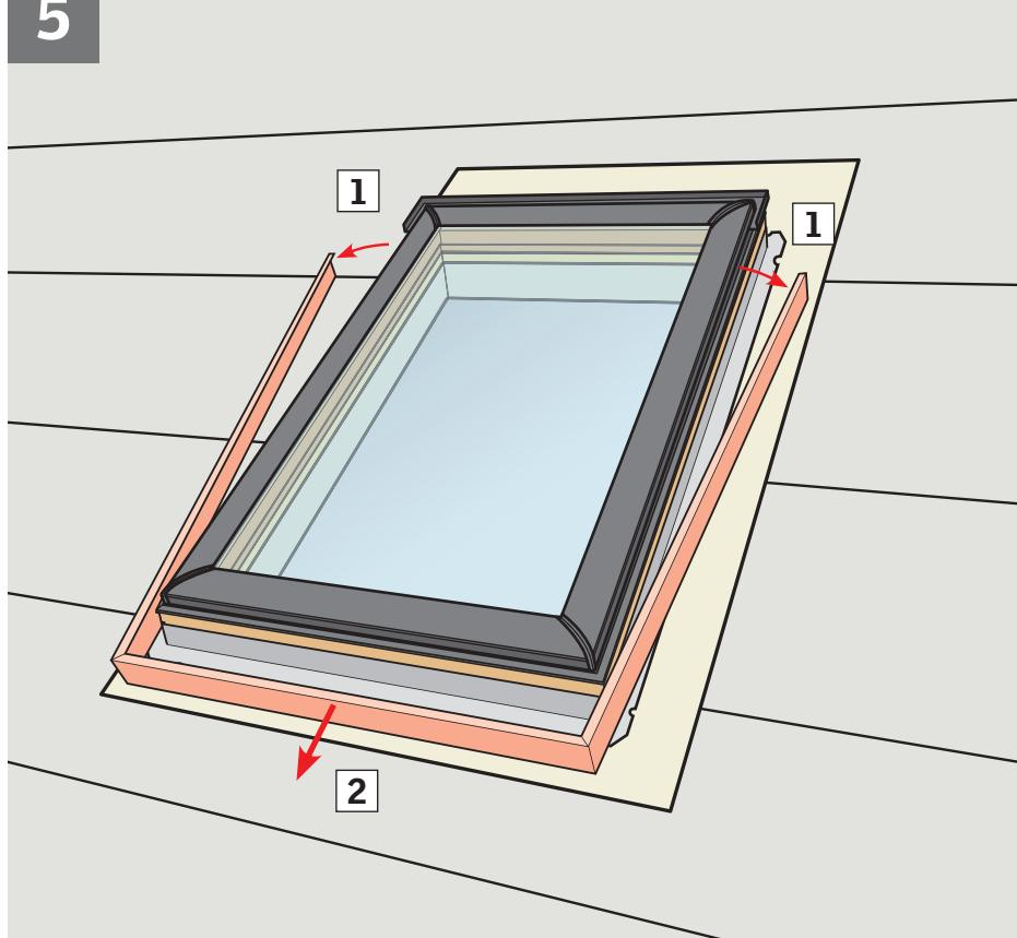
**ENGLISH:** To properly install VELUX adhesive skylight underlayment, remove cladding as shown.
