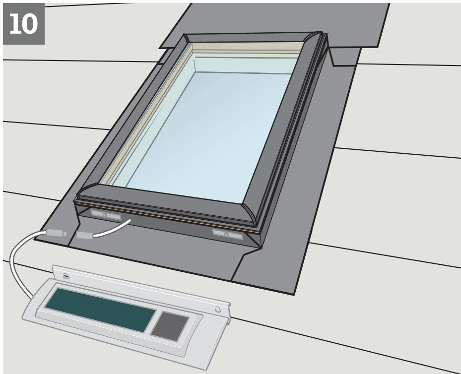
**ENGLISH:** You are now ready to install the flashing. If the flashing is not to be installed immediately, install solar panel and reinstall cladding.
