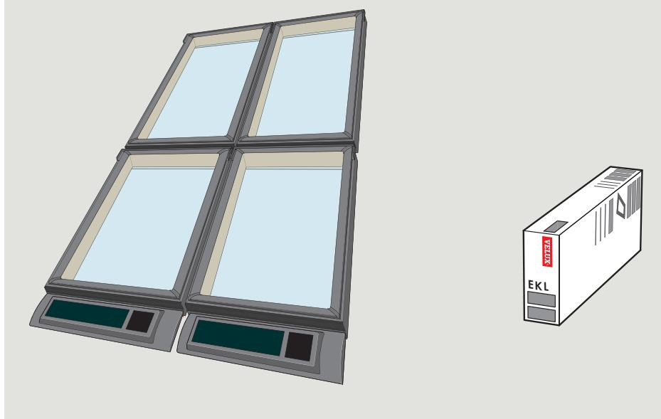
**ENGLISH:** In combi-flashing applications, VSS can only be installed at the bottom row.
