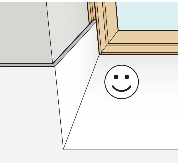
**ENGLISH:** If the drywall is not installed tight into the finish groove, add on-site insulation and trim for finished appearance and to prevent conditions that may contribute to condensation.
