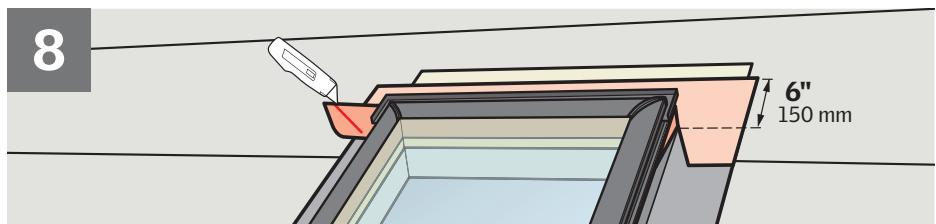
**ENGLISH:** Wrap the top frame and corners of the skylight with VELUX adhesive skylight underlayment and create proper water-shedding lap.
