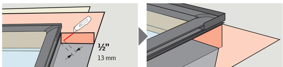
**ENGLISH:** To allow for proper drainage, interweave VELUX adhesive skylight underlayment as shown in 9a for new construction applications. For retrofit applications, interweave VELUX adhesive skylight underlayment as shown in 9b.
