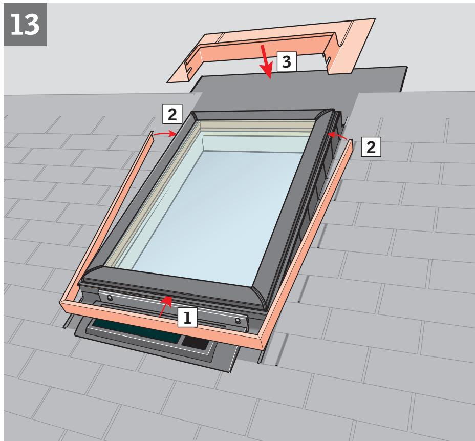
**ENGLISH:** Reinstall cladding (1), (2) and continue installation of flashing (3).
