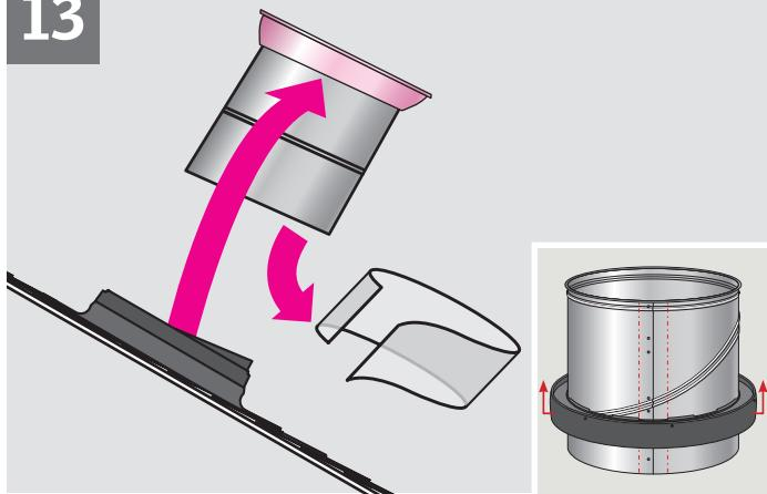
**ENGLISH:** Install the pivot ring on the upper elbow and remove the protective film.
