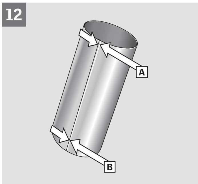
**ENGLISH:** Remove protective film and assemble the straight tunnel sections to go outside the upper sections and inside lower sections. At upper end of tunnel sections, align the notches to create a wide tunnel opening **A** and at bottom of tunnel sections, align the notches to create a narrow tunnel opening **B**.
