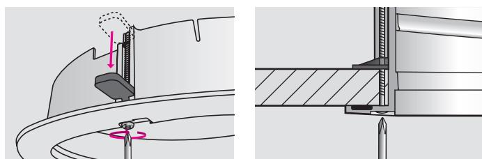
**ENGLISH:** Rotate the plastic "plates" into hidden position and insert and secure the ceiling ring, insuring a tight joint between the ceiling ring and the ceiling.
