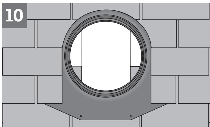
**ENGLISH:** Reinstall roofing material over the flange. Leave a  $5/8"$  (15 mm) channel for water to run off. Optional turret extensions ZTA are available where domes need to be elevated by  $6\frac{1}{2}"$  (165 mm) or  $9"$  (230 mm).
