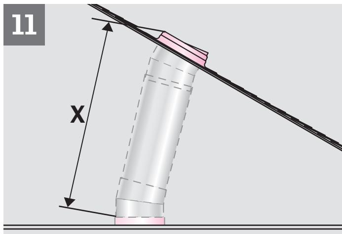
**ENGLISH:** Determine the overall length of the straight tunnel section. Include minimum 3" (80 mm) to overlap the elbows and minimum 1½" (40 mm) for each additional straight tunnel section.
