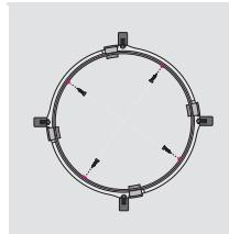
**ENGLISH:** Secure tunnel assembly to ceiling ring with four of the  $\frac{3}{8}$ " (10 mm) screws provided.
