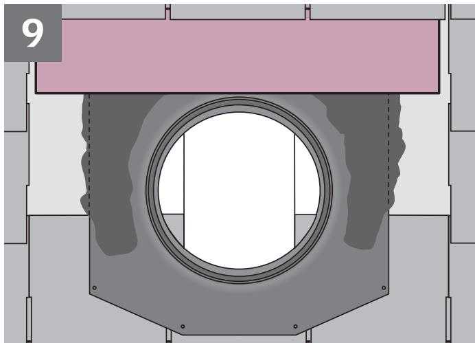
**ENGLISH:** Overlap the top of the flange with underlayment to allow for proper drainage.
