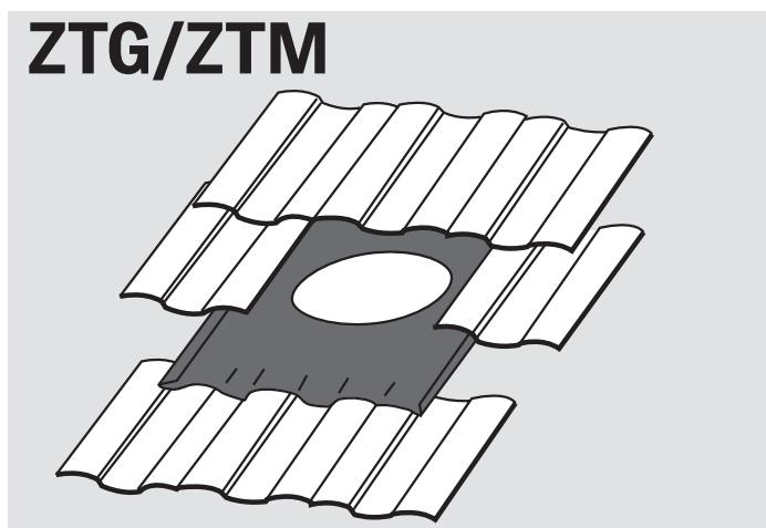
**ENGLISH:** Sun Tunnel tile roofing - Refer to tile kits ZTG/ZTM for installation in tile roofing.
