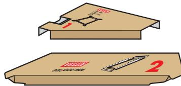
**English:** The sash may be removed to simplify installation. Open sash completely. Press in push button, e.g. with a screwdriver. Remove transportation batten.
