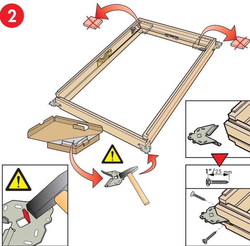
**English:** Remove transportation blocks between sash and frame. Flatten tabs on corner brackets with a hammer and attach the corner brackets with screws provided.
