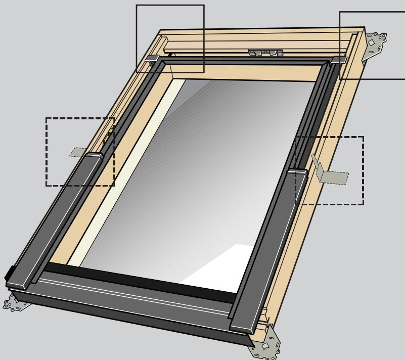
**English:** Secure top brackets fully with  $3\frac{1}{4}$ " (80 mm) screws in the round holes. For long windows secure center mounting bracket with two screws.
