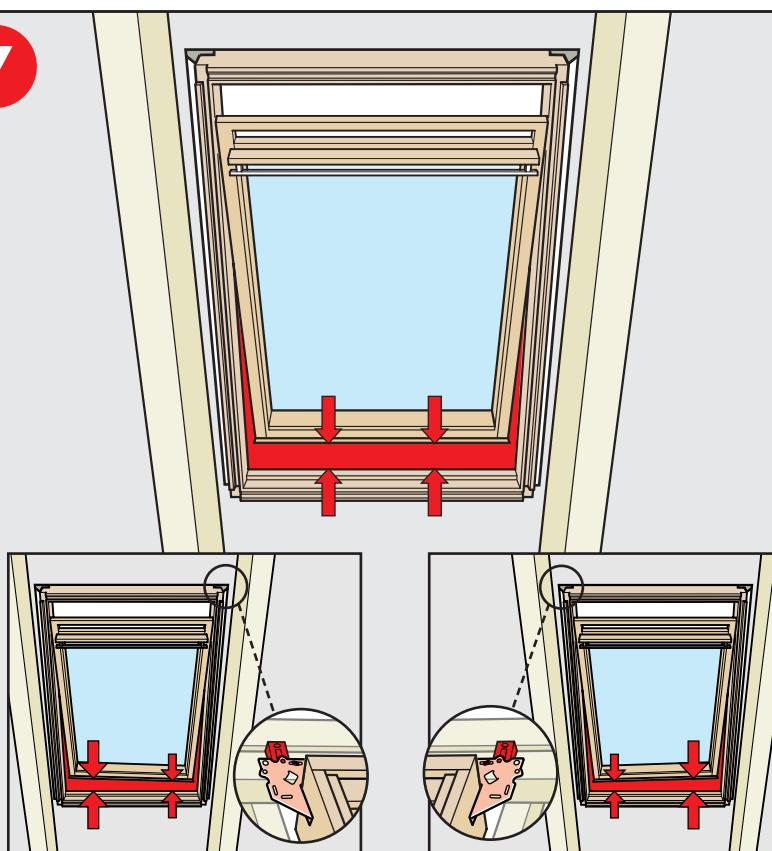
**English:** If uneven rafters cause the frame to twist, adjust using the wedge supplied to ensure an even gap between bottom frame and bottom sash.
