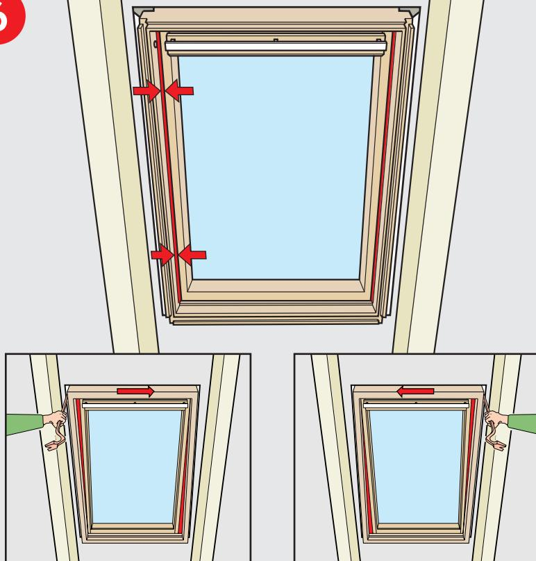
**English:** Adjust window to ensure that the distance between frame and sash is parallel along each side.
