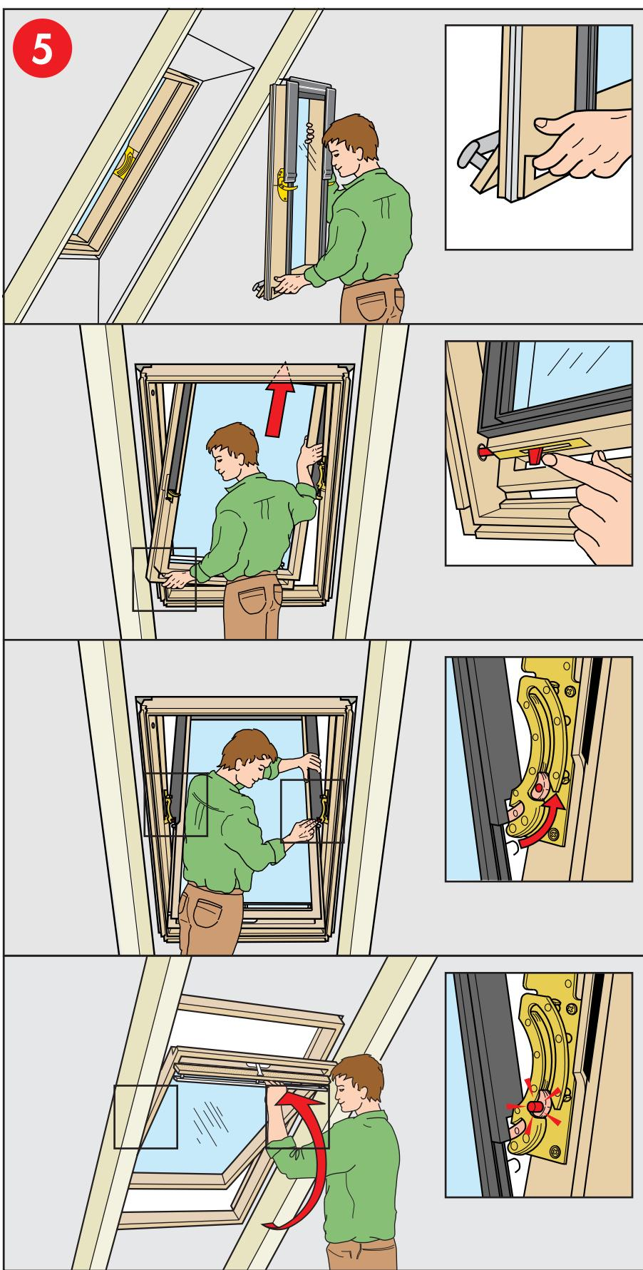
**English:** Replace sash, if removed earlier. The push button is automatically released when the sash is rotated to the closed position.
