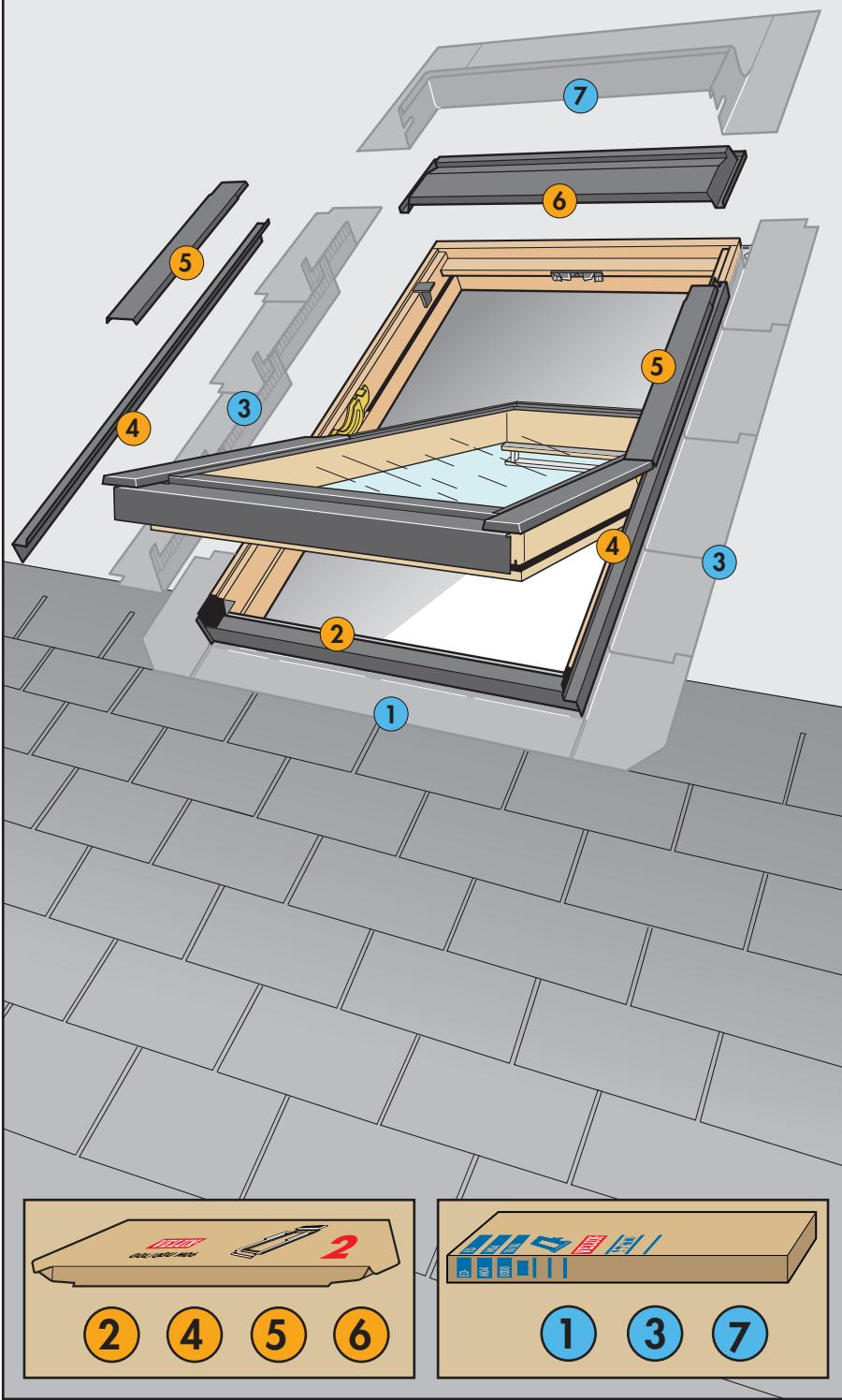
**English:** When fitting flashing and covers, use the instructions supplied with the flashing. If flashing is not to be installed immediately, fit the covers (2, 4, 5, 6.1 and 6.2) supplied with the window.
