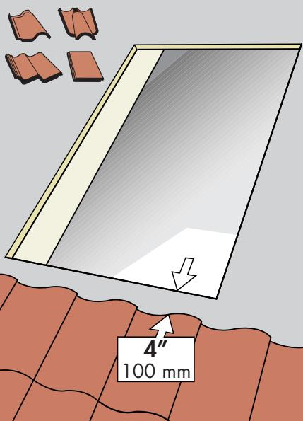
**English:** Attempt to position the rough opening (W x H) in relation to the roofing material in tile roof applications. A full course tile below rough opening will ensure ease of installation and proper performance of EDH/EDW sill flashing.
