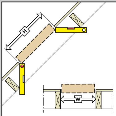
**English:** The rough opening provides the dimension of the opening in the roof deck. When positioning top and bottom headers allow room for vertical and horizontal soffits if necessary.
