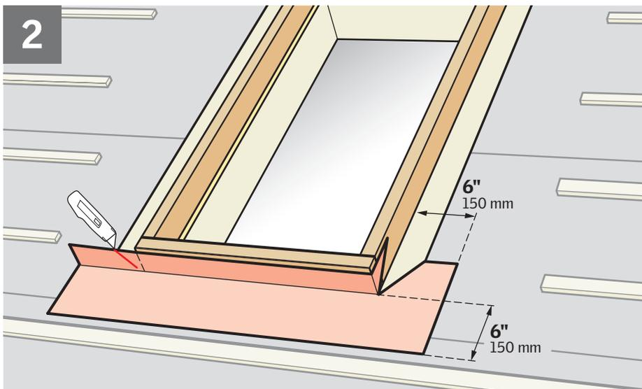
**ENGLISH:** Peel off backing from VELUX adhesive skylight underlayment prior to applying it to roof decking and skylight curb. Ensure that surfaces are clean, dry and free of debris. Wrap the bottom and the corners of the curb with the underlayment and create water-shedding laps over roofing underlayment.
