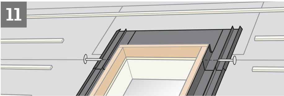
**ENGLISH:** Install and attach saddle flashing to curb with roofing nails as shown.
