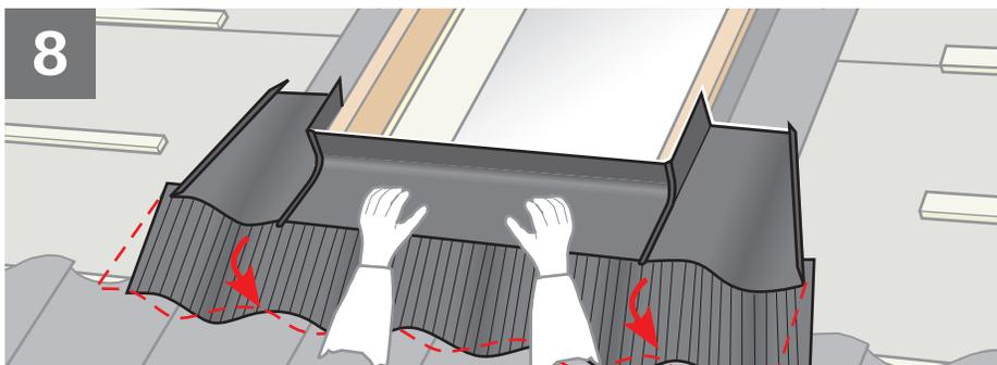
**ENGLISH:** Remove sill flashing section and bend the apron down as shown. This will ensure that the apron lies tightly against the roofing material.
