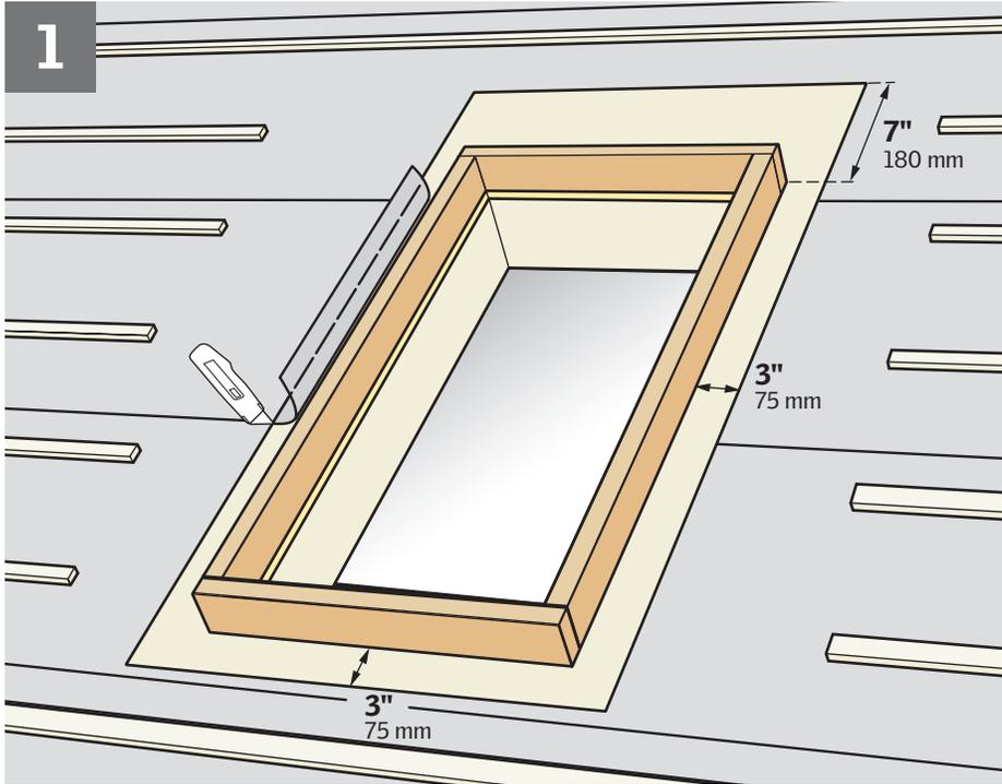
**ENGLISH:** To ensure waterproofing, skylight curbs should be completely wrapped in VELUX adhesive skylight underlayment before installing the flashing.
