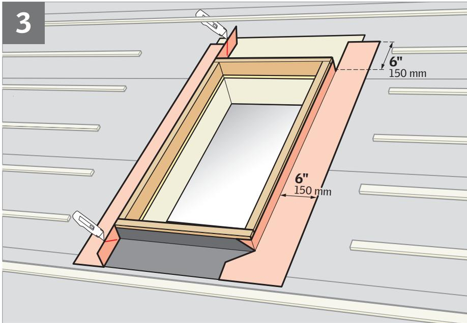
**ENGLISH:** Wrap the sides and the corners of the curb with VELUX adhesive skylight underlayment and create water-shedding laps over roofing underlayment.
