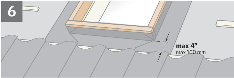
**ENGLISH:** To support the sill flashing section, install roofing material up to bottom curb as shown.
