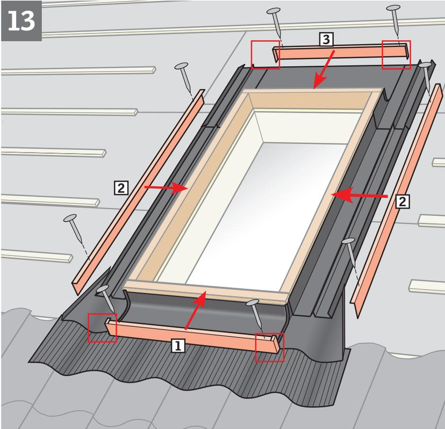
**ENGLISH:** Cut and bend the bottom and top counter-flashings as shown. Attach all counter-flashings to curb with roofing nails.
