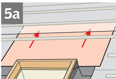
**ENGLISH:** To allow for proper drainage, interweave roofing underlayment as shown in 5a for new construction applications. For retrofit applications, interweave roofing underlayment as shown in 5b.
