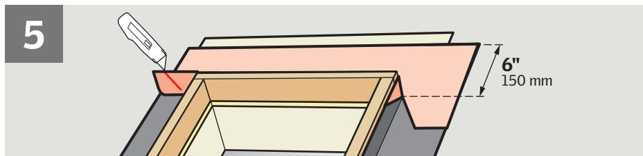
**ENGLISH:** Wrap the top and the corners of the curb with VELUX adhesive skylight underlayment and create proper water-shedding lap.
