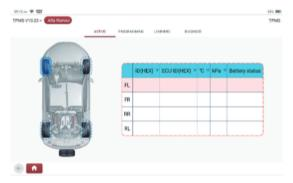
b) Programming: with this function, sensor data can be programmed to a blank THINKCAR sensor to replace one that is low on power and is not working properly. Three sensor programming methods are provided: automatic, manual and activation copy.
