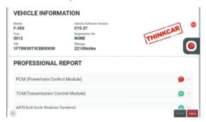
B. System Scan: what systems the vehicle is equipped with are automatically scanned.
