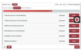
C. Selection scanning: scan the manually selected vehicle electric control system.
