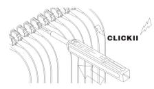
Be careful not to actuate the trueCLEAN on an angle while inserting into the adapter.
