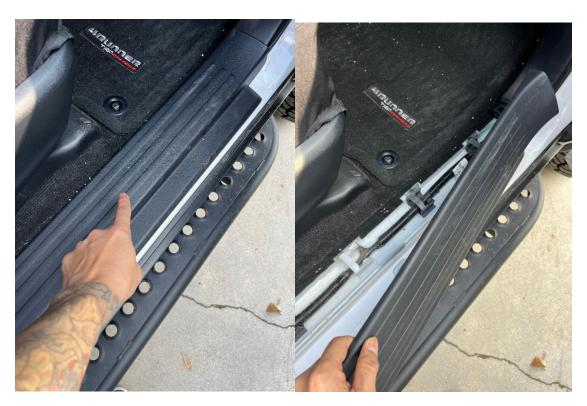
2. Next remove trim panel, making sure to first remove the plastic retaining nut. This can most easily be done by using small needle nose pliers and slightly turning
