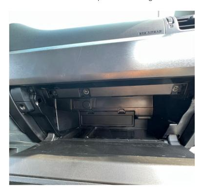
12. Now the dash / glove box is ready to be removed. You will either use the top and right side or left side to grab the whole glove box area and pull it off with force as there are little pink retaining clips are holding it on. When removed, lay on floor or swing out of the way to expose the 4X4 computer module behind the dash.
