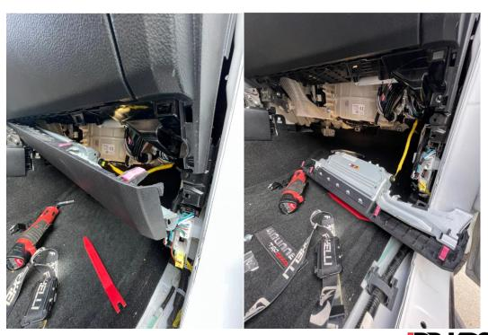
9. Next, remove the 10mm bolt on the right side of the exposed dash (bottom right corner, you will see it once removing the previous panel / airbag bracket)
