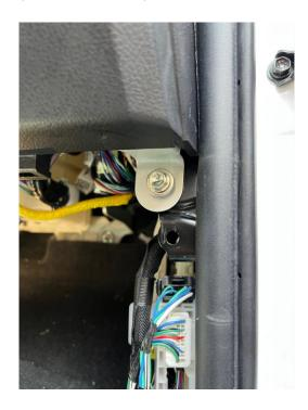
8. Now, pull away the bottom panel / air bag bracket from the lower part of dash (**Note**. start from right to left) - as you are pulling it off making your way to left side, be aware of the metal bracket/hook that connects this airbag bracket to the upper dash bracket. Once removed just lay in it on the floor.
