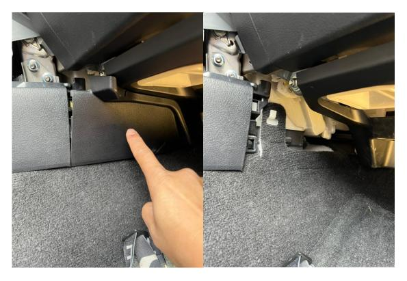
6. Next, remove little plastic trim on left side under the glove box. When removed it will reveal a 10mm - remove that bolt and the other 10mm bolt right below it.
