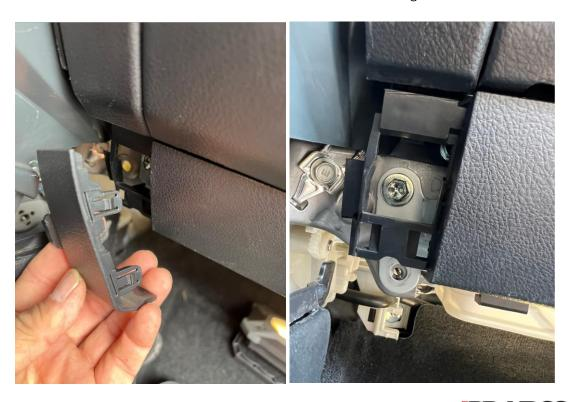
7. Next, remove the 10mm bolt on the opposite side of the dash from the previous bolt (close to the door)
