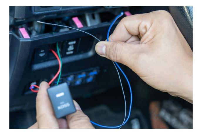
**Step 11:** T-Taps Review (Check back for vehicle make instructions) To enable the lights you will use the provided T-Taps to tap into a neighboring OEM switch. I recommend that you T-Tap into the front defrost switch. Please review how T-Taps work:
