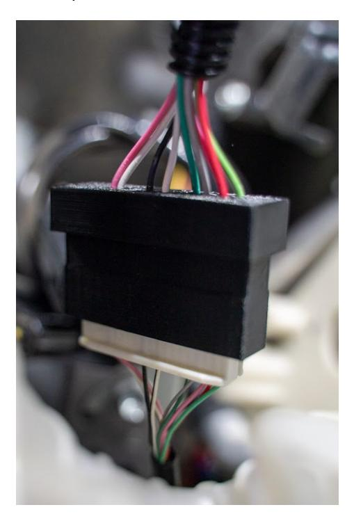
**Step 3:** Harness to KDSS ECU Now plug the white connector on the harness back into the factory KDSS ECU module.
