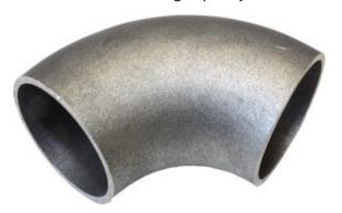
Lockinex™ welding elbows for handrails and balustrades are ideally suited for tubular constructions where aesthetics are of prime importance. The use of these welding elbows enables tight bends and curves to be obtained even on large diameter tubes and resolves the problem of either sharp mitred edges or distortion, which occurs on tubes when radiused. They provide a neat safe joint which is permanent and strong.
