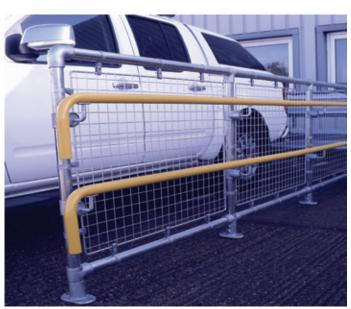
With a guardrail (1100mm high), a DDA handrail (900mm high) can be suspended from the vertical posts. This format complies with regulations for safety guardrails and building regulations for the provision of a handrail system.
