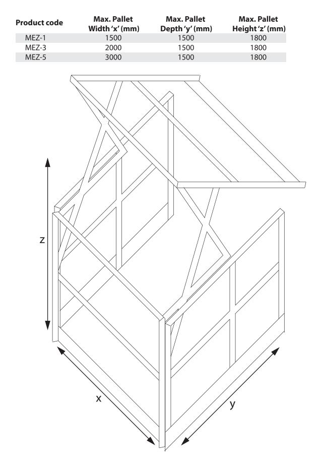
Kits are supplied with components ready to assemble and install with the above finished dimensions. However, if different dimensions are required the horizontaol rails etc. can simply be cut down on site to create desired dimensions.
