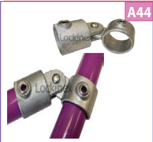
A flexible variable angle connector. Used for an angled top rail connection to a post. Use if the angle required is not known. Also used as bracing struts for racking etc. Reducing combinations are available throughout the size range.
