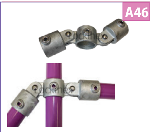
A flexible variable connection used for an angled lower rail(s) joint to a post. Changes horizontal rails to angled rails at top of ramps/stairs. Also as bracing struts for racking. Reducing combinations available throughout the size range.
