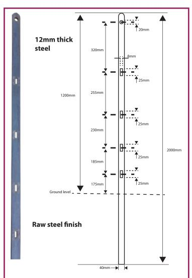
40x12mm estate fencing post, 2000mm long. Top hole to accept 20mm round bar. 4x lower holes to accept 25x8mm round bar. Rounded post top. Raw steel finish.
