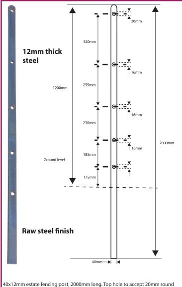
40x12mm estate fencing post, 2000mm long. Top hole to accept 20mm round bar. 4x lower holes to accept 16mm round bar. Rounded post top. Raw steel finish.
