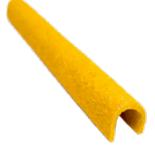
Hi visibility yellow non-slip GRP ladder rung covers suitable for rungs with 20-25mm dia. Fix to ladder rungs using a PU230 adhesive which acts as an adhesive and a packer/filler.
