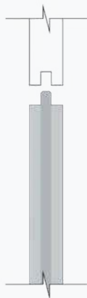
Internal lining end match profile not to scale
