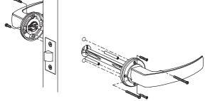
To attach furniture to the door fit the threaded spindles to one side of the backplate first then insert the square spindle with the scalloped side facing the grub screw in the handle. Then offer up to the door and fit the other handle. Screw the machine screws into the threaded spindles. Tighten the grub screws in the handles. Then add extra wood screws for strength.
