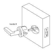
7. Remove the o-ring from the spindle. Insert the spindle into the latch so an even amount protudes on each side of the door and slide the o-ring back onto the spindle. Insert handle 'A' with rapidFIT® attached onto the spindle in the 48mm hole and press against the door.
