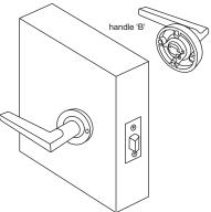
Note: The grubscrews may need a re-tighten after a bedding-in period. We recommend medium strength thread-lock to be used.
