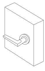
6. Screw the rose cover onto the handle and tighten the grubscrew on the side of the lever onto the spindle. For the square rose (Futura Elite) press on the rose cover and tighten the grubscrew on the side of the rose.
