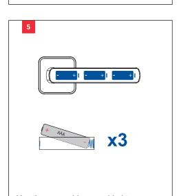
Use the screw driver provided to unscrew the battery cover located in the inside handle. Then install the batteries (negative terminal going first). Cover the batteries.
