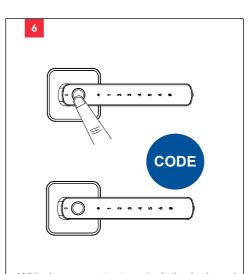
With door open try to unlock the lock and make sure the installation was successful. In factory default mode, the lock will unlock with 123456# or any finger print.
