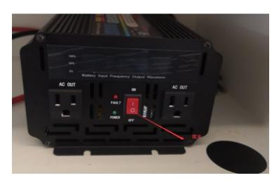
Looking from above picture, there are two switches for the inverter, our engineer suggest only use the switch on the control panel as before and keep the switch closed on inverter itself.
