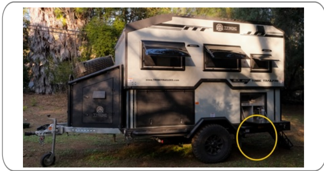
Location of black and gray water dump valve
