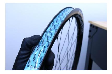
**Step 6:** Once the tape has reached its starting point, continue working the tape around past the valve hole once again. Once the tape is approximately five inches past the valve hole, cut the tape and press the end down firmly to seal the tape on the rim. We like to cut the end of the tape at a 30-45° angle. There should be about a 10 inch long section of tape around the valve hole that is overlapping, two layers thick. The remainder of the tape only needs to be one layer thick.
