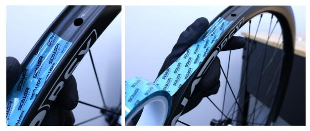
**Step 5:** Continue to work the tape around the rim, passing the valve hole. Work out as many air bubbles as possible along the way (a few small air bubbles after the tape is applied will not be detrimental to the tape's performance). Apply pressure from the center of the rim bed and work your way up to the two sidewalls as you go. The tape should be contacting all of the rim bed's surface area after it is applied.
