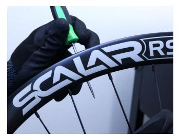
**Step 10:** Using a 4.5 to 5.5 mm diameter phillips screwdriver or ball nosed allen wrench, slowly enlarge the hole made by the pick. Other tools may also be used. The goal here is to make a 4.5 to 5.5mm diameter hole that the valve can push through.
