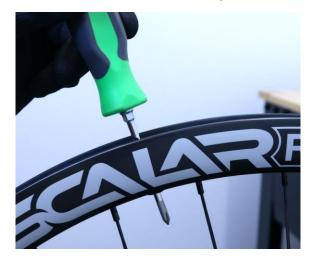
Step 11: Disassemble the valve, laying out the stem, o-ring, nut, and cap.
